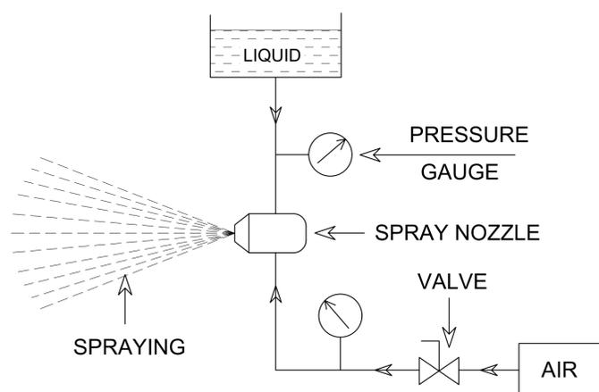
3 ) **Siphon Method** : In this method of liquid supply, The liquid is feed by the suction of liquid from a certain siphon height of liquid by pressurized Air ,This method is basically used where liquid tank and motor pump is not available for liquid feeding .
